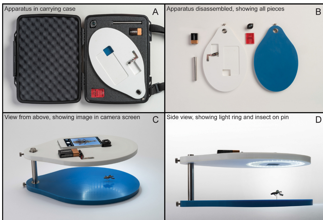
FIGURE 2.1: Photographs of the device developed for capturing high-quality images of kissing bugs. (A) and (B) top view of the device; (C) and (D) lateral view of the device with the lighting ring and an insect (not a triatomine) placed on the pin.
