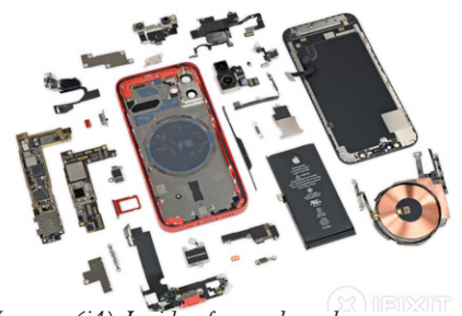
Image: (i4) Inside of a modern day smartphone. Note the copper colored wireless charging component, which basically is an electromagnet.
