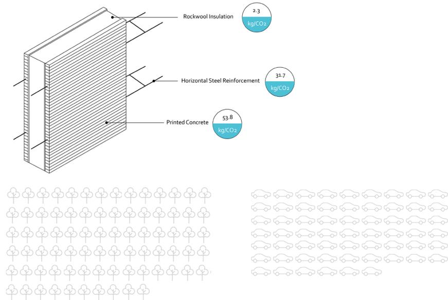
Figure 5.03 Blue Planet Wall Section
