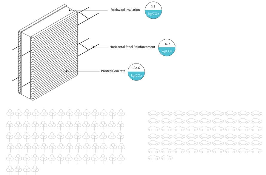
Figure 5.01 Laticrete Wall Section
