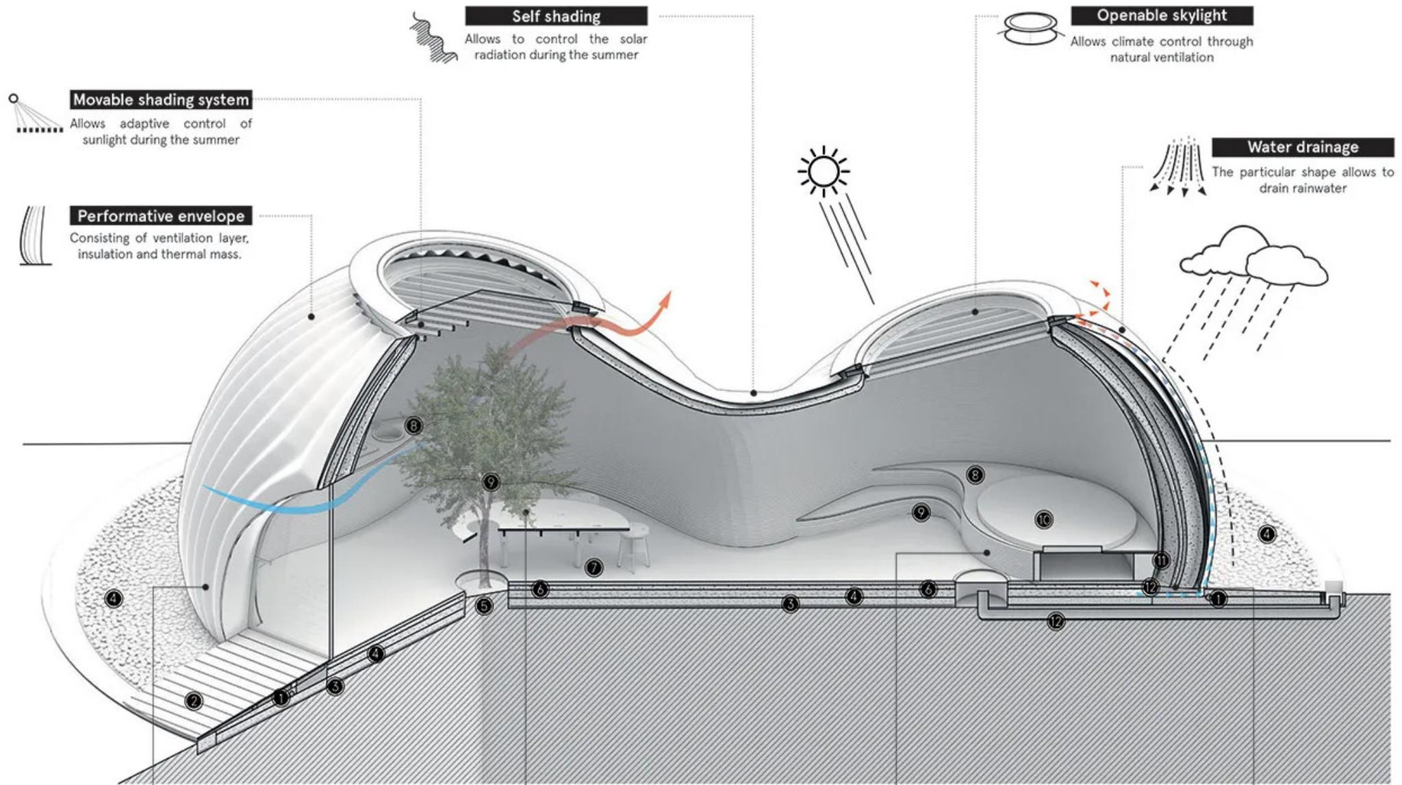
Figure 3.03 Detailed axonometric section of the TECLA prototype
