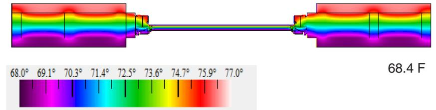
Figure 7.16 3D printed window detail summer
