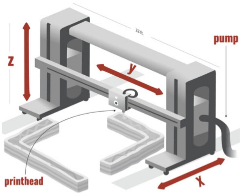
Figure 2.00 Gantry System Diagram
