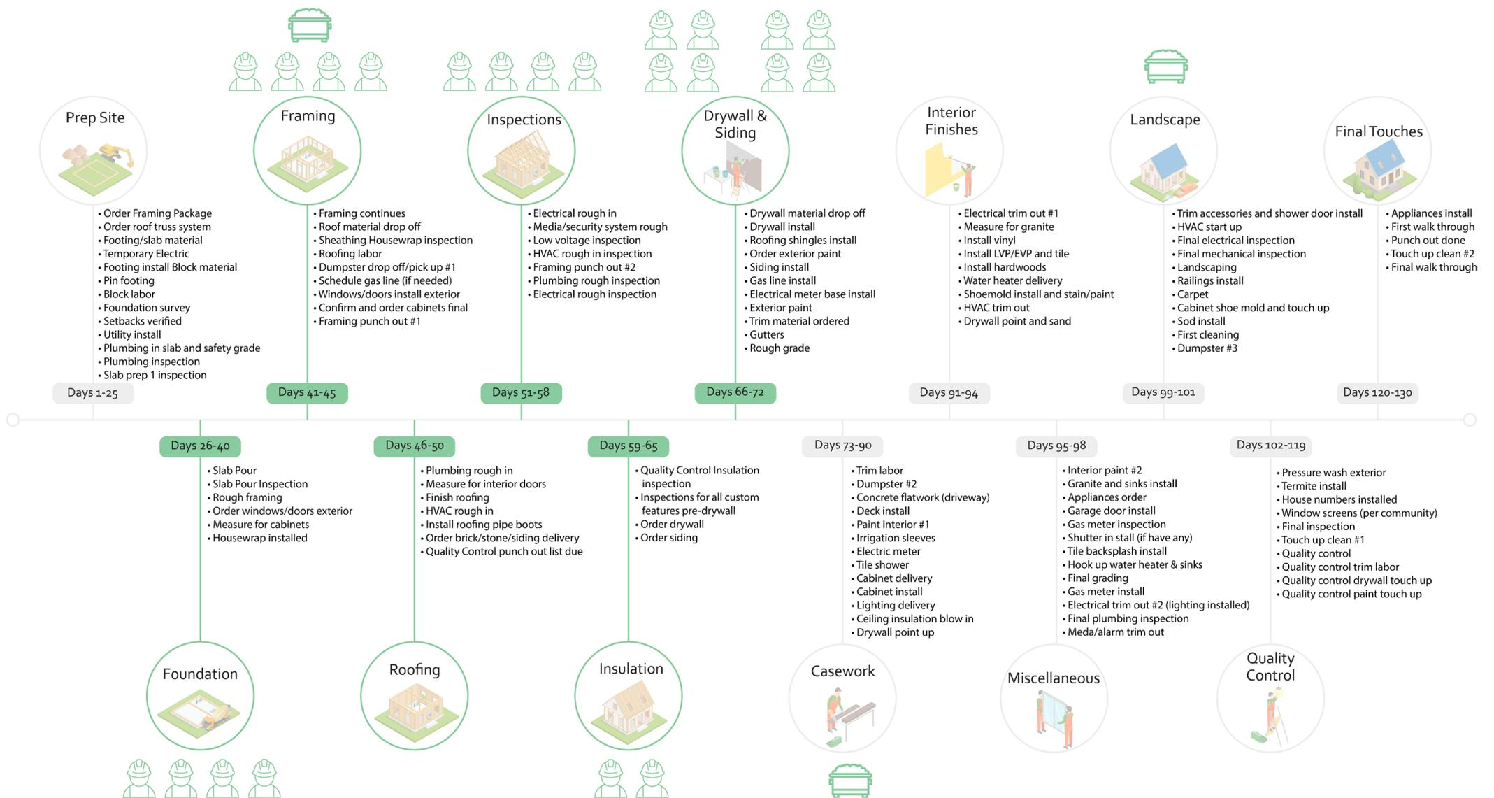
Figure 5.06 Typical Wood Frame Timeline
