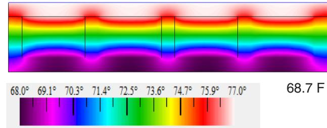
Figure 7.08 3D printed wall summer
