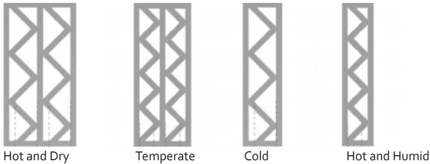
Figure 10.00 3D printed thermal resistant layers per climate conditions
