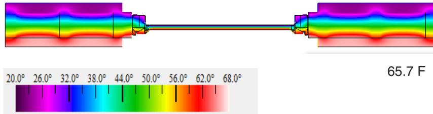
Figure 7.14 3D printed window detail winter
