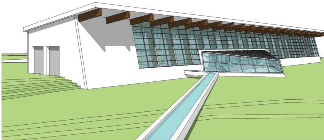
The building uses the section from the earlier study adding the benefit of operable windows on the south facing glazing. On the north wall there are opaque insulated panels that open to allow for natural ventilation.
