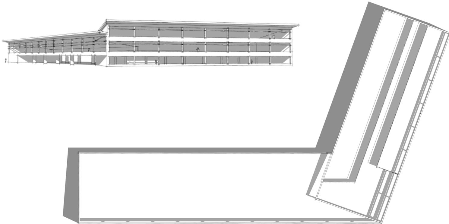
This attempt featured site lines to the wetland and the river. The West half of the building is raised and is positioned over the reservoir that is used to irrigate the site
