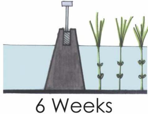
Gradual flooding protects the liner and allows plants to become acclimatized as they begin to grow.<sup>1</sup>
