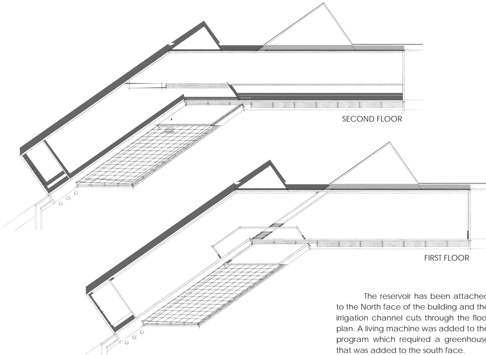
The reservoir has been attached to the North face of the building and the irrigation channel cuts through the floor plan. A living machine was added to the program which required a greenhouse that was added to the south face.
