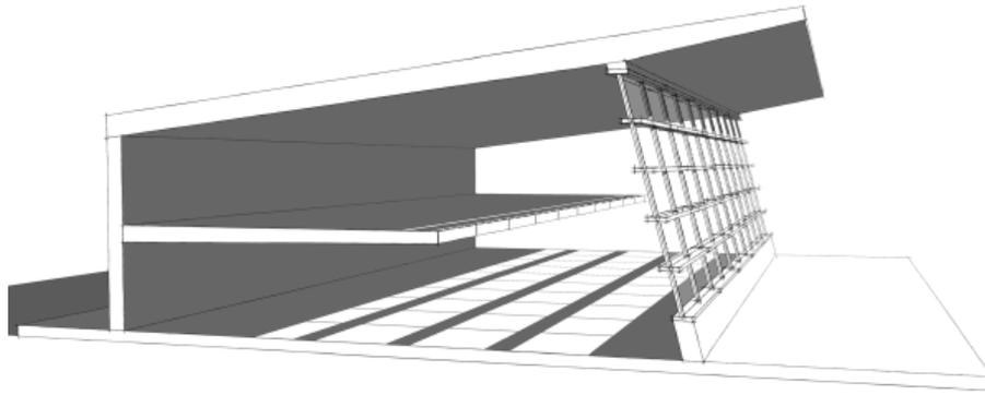
This is a study of a more ecological section for future attempts at the project's form. It is designed specifically so that the section protects the glass from the summer sun while allowing the winter sun to penetrate deep into the building providing for passive solar heating.
