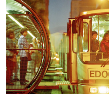
(Upper Left) Tubular stations with loading platforms extended to load and unload passengers onto awaiting bus.
