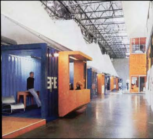
A main street of shipping containers, sheltered by tensile canopies, the unique look at the low cost and energetic space of the shipping container provides a solution for the office space of Clive Wilkinson Architects.
