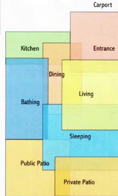
Idealized space diagram developed during the schematic phase of design for the possible flow and layering of space. Includes some additional spaces not included in the final program such as the kitchen and dining spaces.
