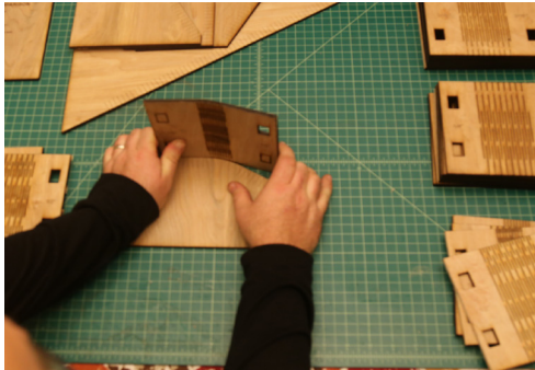
These pictures show a series of strength and flexibility tests on various kerf cuts.
