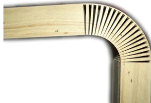
Fig. 17: traditional woodworking kerf or relief cut
