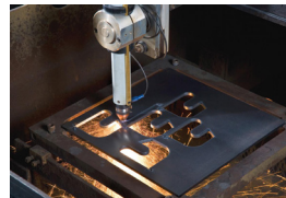
Fig. 23: Plasma cutter, cutting through steel
